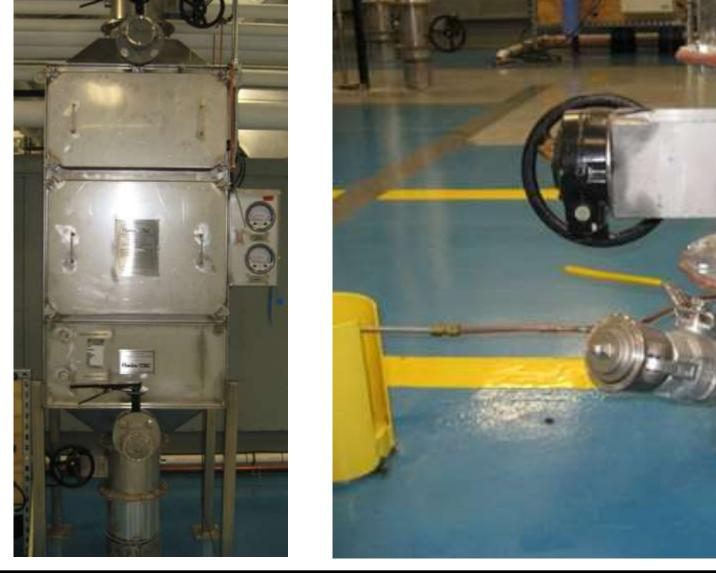
Figure 3. Closed loop system used at BRI (CD gas set-up shown).
