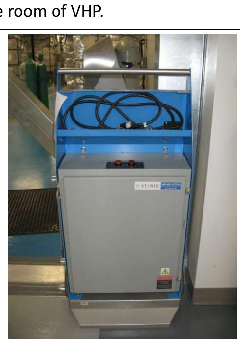
Figure 1. Steris VHP 1000-ARD System with dryer unit and dryer regeneration unit.
