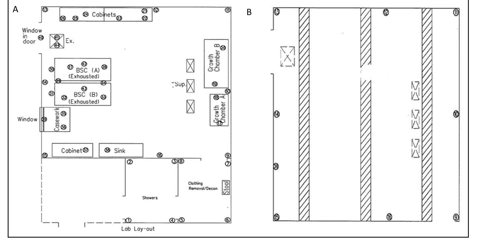
Figure 7. Typical room schematic of BI and CI placement in a BSL-3 lab during cycle optimization. The figure on the left shows BI and CI placement in the room (A). The figure on the right shows BI and CI placement above the false ceiling (B)
