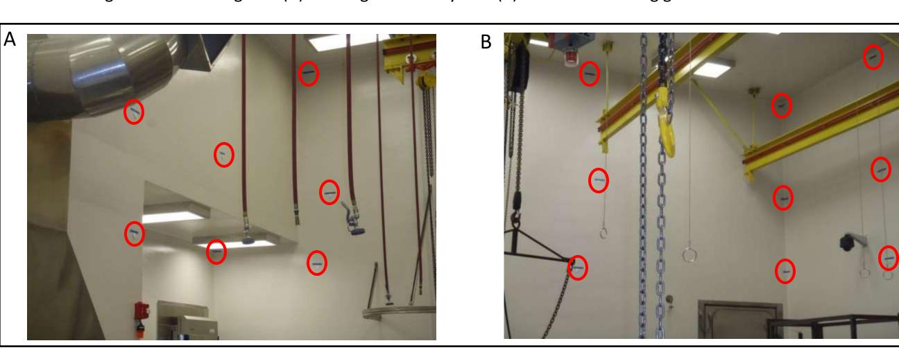
Figure 6. Biological (BI) and chemical (CI) indicator pairs hung throughout the room with blue painter's tape. During cycle optimization, BI and CI pairs are hung in predetermined spots throughout the room and in any hard-to-reach places.
