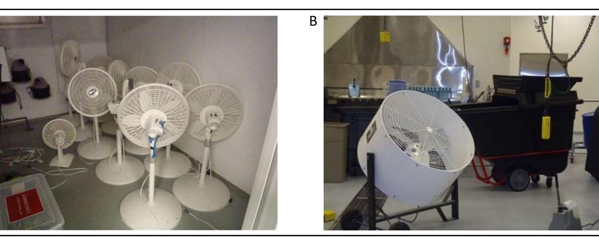
Figure 5. Oscillating fans (A) and large stationary fans (B) used at BRI during gas decontamination.
